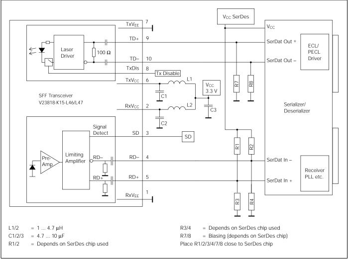
Values of R1/2/3/4 may vary as long as proper 50  $\Omega$  termination to V<sub>EE</sub> or 100  $\Omega$  differential is provided. The power supply filter-
