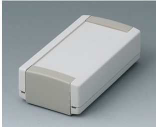
B1040365 TOPTEC 102, Vers. I ABS (UL 94 HB) off-white RAL 9002 4.02"x2.13"x1.18" IP 40
