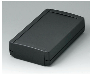
B1075369 TOPTEC 194 F, Vers. I ABS (UL 94 HB) black RAL 9005 7.64"x4.53"x1.81" IP 40
