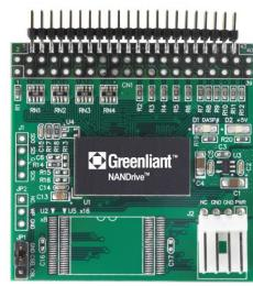
Figure 2: NANDrive Evaluation Board, 44-pin Connector
