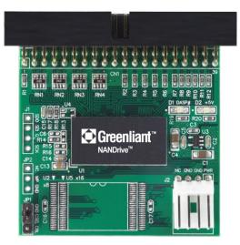
Figure 1: NANDrive Evaluation Board, 40-pin Connector
