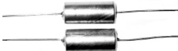
The Type THF is ideal for use in switching regulators and high frequency power supplies because of its high ripple current and low ESR capabilities. It is an axial lead solid tantalum capacitor constructed with a rugged hermetically sealed metal case, insulated with an outer polyester wrap. The THF assures a small case size for high capacitance, and is extremely stable over the rated temperature range.
