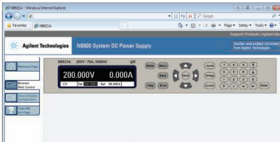
Figure 3. N8900 Series web graphical user interface for remote access and control of the power supply
