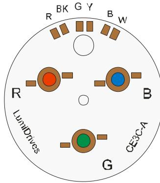
**NOTE**- At the side of this drawing are the recommended wire colours to use when wiring this product. The pads are marked on the **Colour Engine 3** with the correct wire colour to use. **R**= RED, **G**= Green, **B**= Blue, **BK**= Black, **Y**= Yellow and **W**= White. The polarity key is used to determine the positive and negative channels on the **Colour Engine 3**
