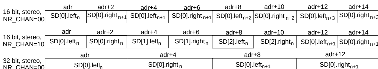
Figure 2: Examples of Audio Out Memory DMA Formats
