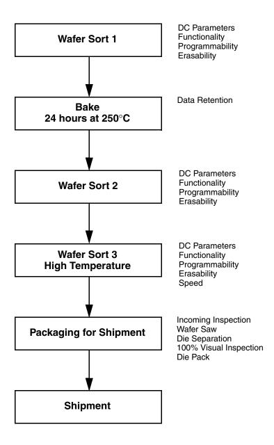
Figure 1. AMD KGD Product Test Flow
