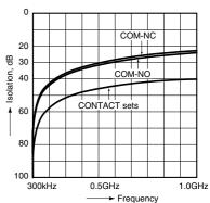
1-(2). High frequency characteristics (Impedance  $75\Omega$ )
