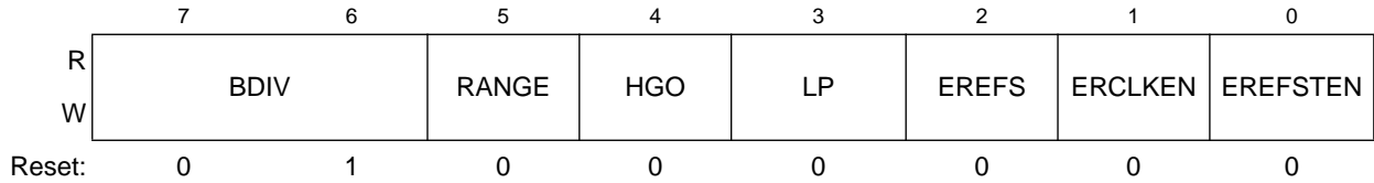
Figure 8-4. MCG Control Register 2 (MCGC2)
