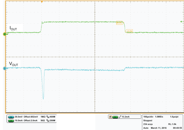
Figure 29. Load transient ( t_{rise} = 5 \mu s )
