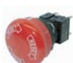
Round Medium 40 mm dia., Push-lock turn-reset A165E-S
