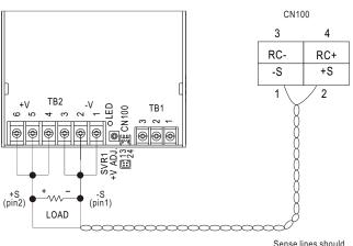
Sense lines should be twisted in pairs
