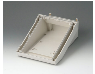
B4016317 DATEC-TERMINAL M, Vers. III ABS (UL 94 HB) off-white RAL 9002 6.61"x10.71"x3.98" IP 54 opt.
