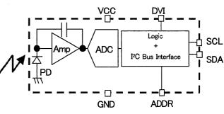
\* Initial reset is necessary on power supply sequence. (More than 1us)
