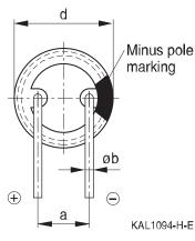
Minus pole The series B41898 has no marking sleeve nor minus pole marking, the positive pole is marked on the aluminum
