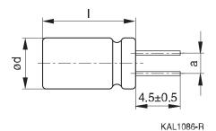
10 × 16 5.0  $10 \times 20$ 5.0  $12.5 \times 20$ 5.0  $12.5\times25$ 5.0 16 × 20 7.5  $16 \times 25$ 7.5  $16 \times 31.5$ 7.5  $16 \times 35.5$ 7.5 7.5  $18 \times 20$  $18 \times 25$ 7.5  $18 \times 31.5$ 7.5  $18 \times 35$ 7.5  $18 \times 40$ 7.5
