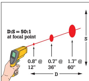
Use the Fluke 68 and 68IS within 8 m (25 ft.) of the intended target. At greater distances, the measured area will be larger (approximately the distance divided by 50).
