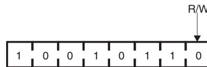
Figure 6. Software Reset Address
