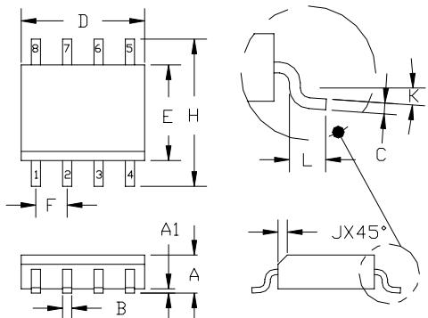
3. MOLDED PACKAGE SHALL CONFORM TO JEDEC STANDARD CONFIGURATION MS-012 VARIATION AA.
