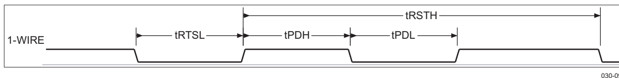
Figure 6-59. 1-Wire Break (Reset) Timing
