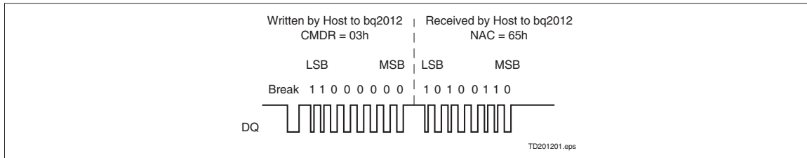
Figure 3. Typical Communication With the bq2012
