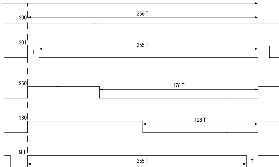
Figure 12-2 PWM output waveforms (POL = 1, active high)
