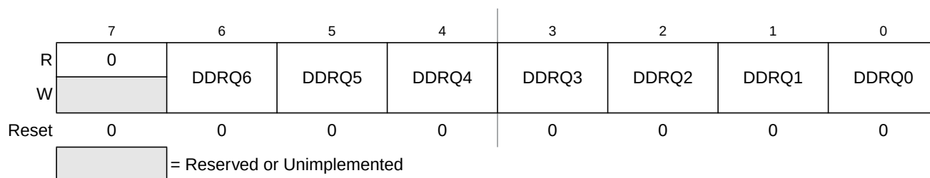
Figure 3-25. Port Q Data Direction Register (DDRQ)
