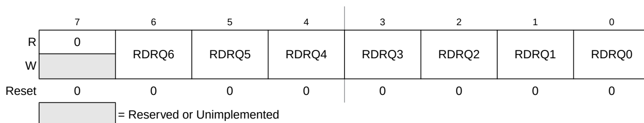
Figure 3-26. Port Q Reduced Drive Register (RDRQ)
