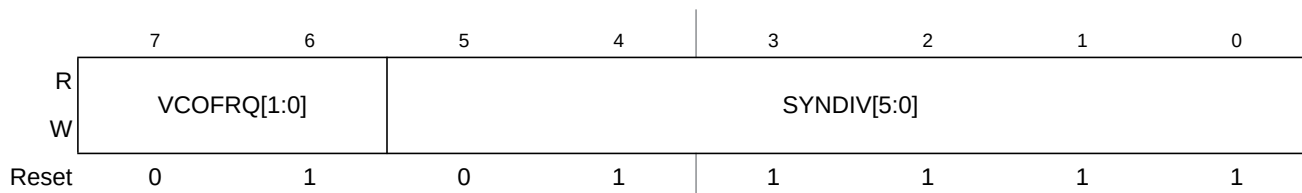
Figure 7-4. S12CPMU Synthesizer Register (CPMUSYNR)
