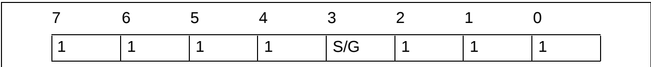
Figure 26 MONITOR Channel on IDP0
