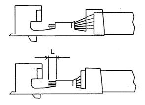
As the insulation stripped length is longer than the specified one, the insulation is inserted into half length of the insulation barrel only, or the dimension "L" is more than 0.6 mm.
