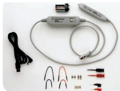
N2793A 800-MHz, 15-V differential probe
