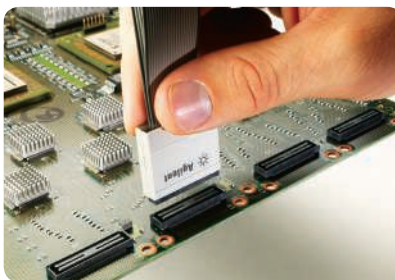
E5385A 34-channel Samtec connector probe
