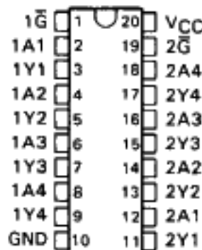
SN54ALS467A, SN54ALS468A . . . J PACKAGE SN74ALS467A, SN74ALS468A . . . DW OR N PACKAGE (TOP VIEW)
