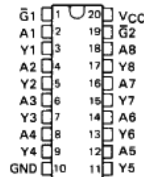
SN54ALS465A, SN54ALS466A . . . J PACKAGE SN74ALS465A, SN74ALS466A . . . DW OR N PACKAGE (TOP VIEW)
