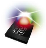
The AS3693B is a 16 cannels high precision LED controller with build in PWM generators for driving external FETs in LCD-backlight panels.
