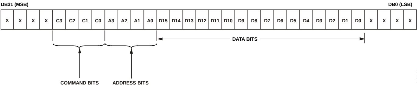
Figure 47. AD5678 Input Register Content for DAC A, B, G, H
