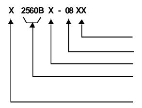
Package: ST: SOIC in TUBE SR: SOIC in TAPE & REEL
