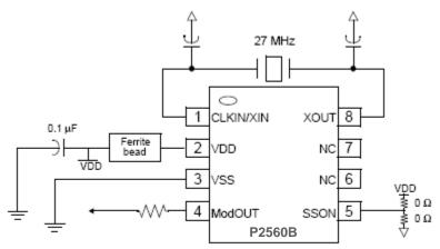
Use either pull-up or pull-down resistors with 0  $\Omega\!.$
