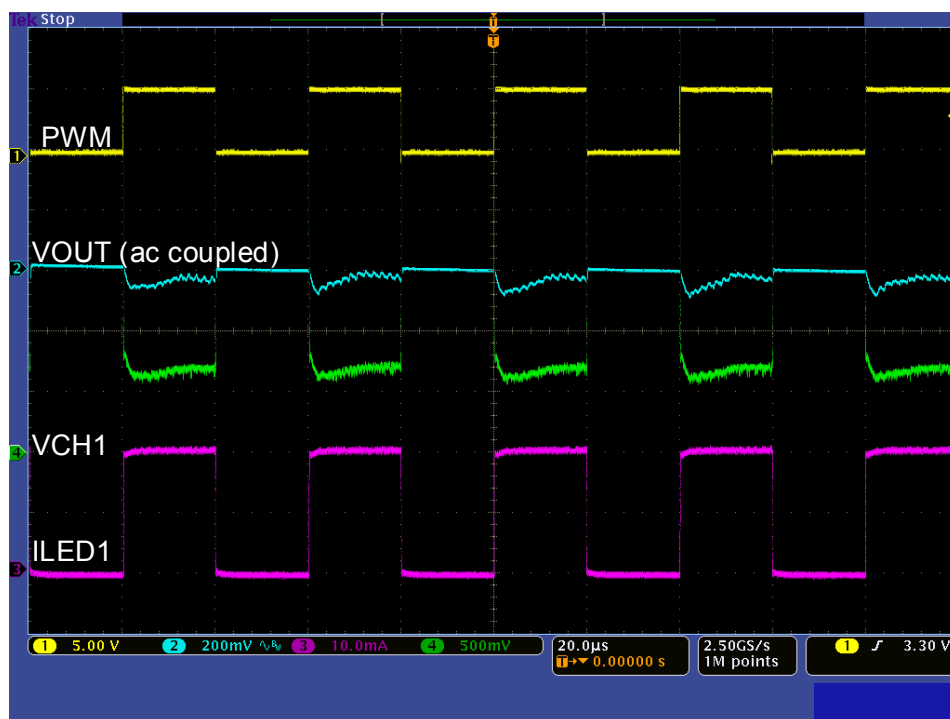
Figure 8. Typical Operating Waveforms (FPWM=25kHz, 50% duty)
