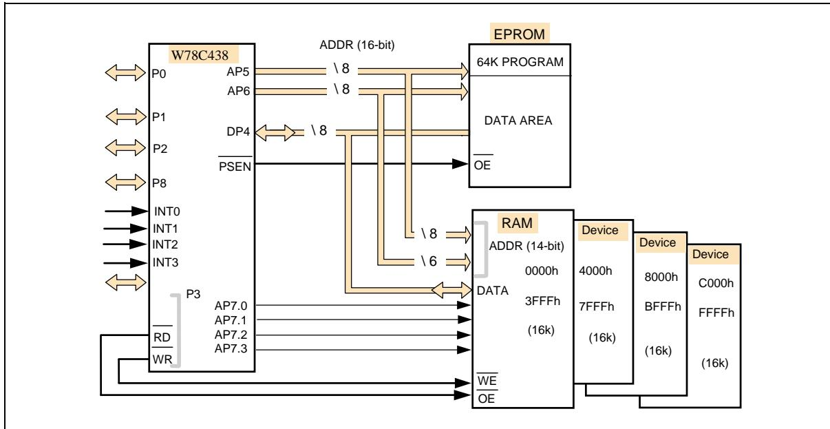
The EPMA register is a nonstandard 8-bit SFR at address 0A2H in the standard W78C32. To read/write the EPMA register, one can use the "MOV direct" instruction or "read-modify-write" instructions. Bits <6:4> of the EPMA register are reserved bits, and their output values are 111B if they are read. The content of EPMA is 70H after a reset. The EPMA register does not support bit-addressable instructions.
