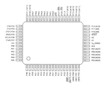
Figure 2.1 (2). Pin Assignment (Flat Package)
