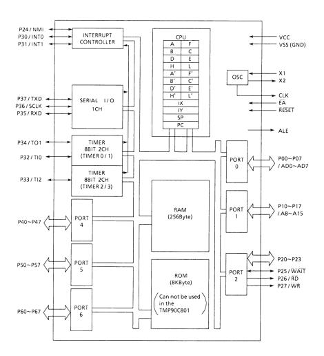
Figure 1. TMP90C800 Block Diagram
