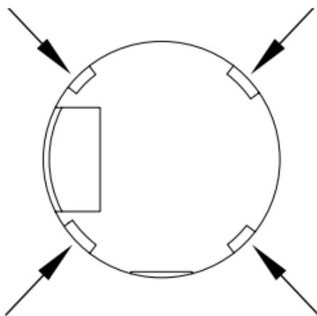
Insert the lithium battery (CR2032) supplied into the battery holder (E), observing the correct polarity (positive pole at the top).
