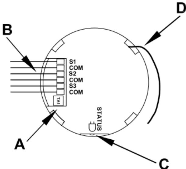
To switch the shutter contact interface to teach-in mode, briefly press the teach-in button (A). The shutter contact interface will then enter configuration mode for 20 seconds; this will be indicated by the
