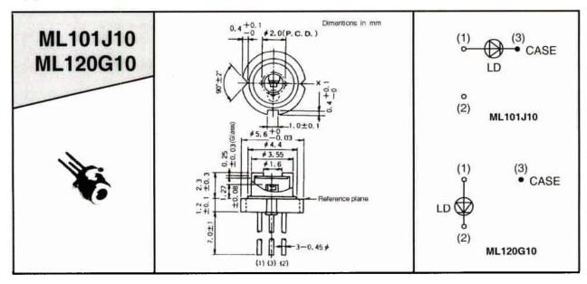
There is no model with a monitor photo diode in ML1XX10 series.
