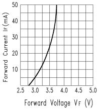
Forward Voltage VF (V) Fig.2 Forward Current vs. Forward Voltage
