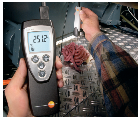
Temperature measurement of ductile materials with the fast-action penetration probe
