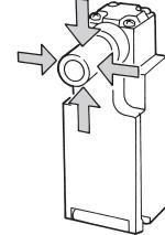
Be sure that the arm lever and door are mounted as shown in the following diagram so that the arm lever and head are not subjected to mechanical stress when the door opens or closes.
