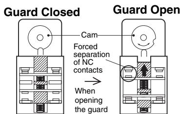
When the guard is opened, the cam that is directly coupled to the shaft rotates to press the Switch in the direction shown by the (vertical) arrow. This action separates the contacts to stop the machine.
