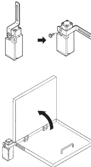
**Note:** Install the arm lever so that it will not rotate more than 180°.
