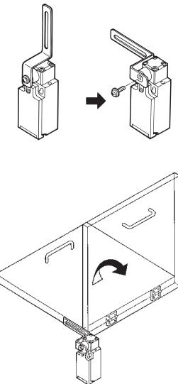
**Note:** Install the arm lever so that it will not rotate more than 180°.
