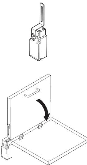
**Note:** Install the arm lever so that it will not rotate more than 90°.
