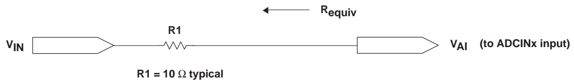
Figure 42. Typical ADC Input Pin Circuit
