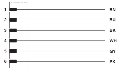
Contact assignment of the DEUTSCH DT04-6P
