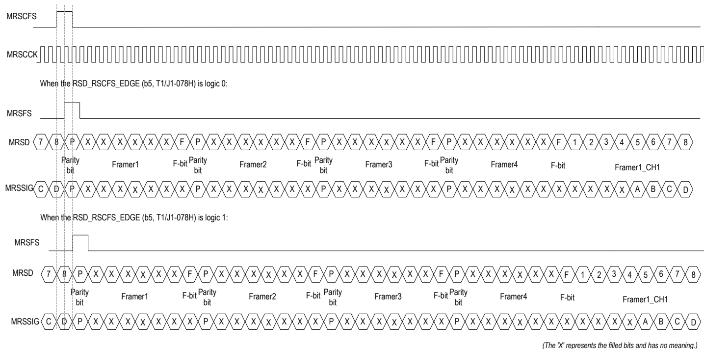
Figure 34. T1/J1 Receive Multiplexed Mode - Functional Timing Example 2
