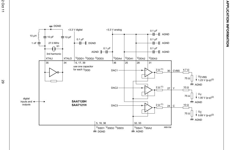
Fig.11 Application circuit.
