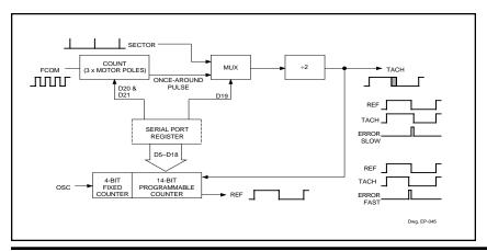
$\frac{\text{desired}}{\text{total count}} = \frac{60 \text{ x f}_{\text{OSC}}}{\text{desired motor speed (rpm)}}$  where the total count (number of oscillator cycles) is equal to the sum of the selected (programmed low) count numbers corresponding to bits D5 through D18.
