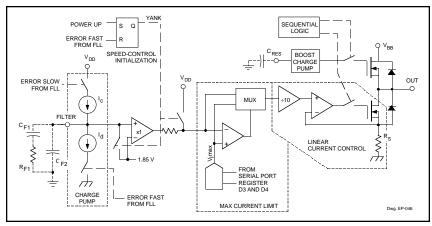
**Speed Control.** The A8902CLBA includes a frequency-locked loop speed control system. This system monitors motor speed via internal or external digital tachometer signals, generates a precision speed reference, determines the digital speed error, and corrects the motor current via an internal charge pump and external filtering components on the FILTER terminal.
