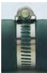
Hose installed with unlined clamp
