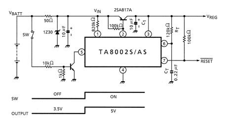
\*: Use an output capacitor C<sub>1</sub> which has a low temperature dependence (such as a tantalum capacitor) . Connect it as close to the IC as possible.
