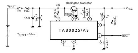
\*: Select a C<sub>2</sub> value according to the working condition - typically above 2000pF.
