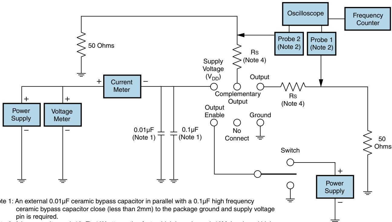
Note 1: An external 0.01μF ceramic bypass capacitor in parallel with a 0.1μF high frequency ceramic bypass capacitor close (less than 2mm) to the package ground and supply voltage pin is required.
