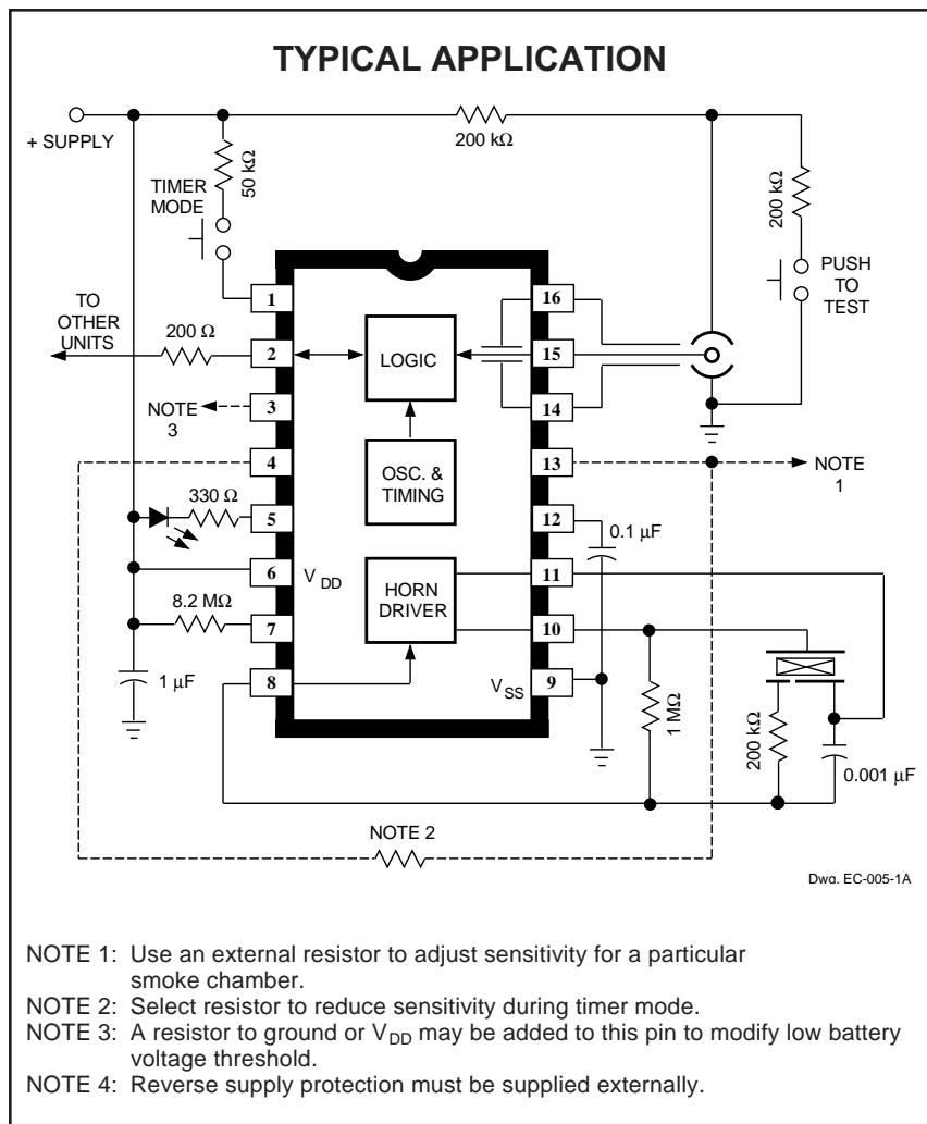
sound their associated horns after a nominal 3 second delay. The LED remains ON when an alarm is signaled from an interconnected unit and a local smoke condition does not exist.
