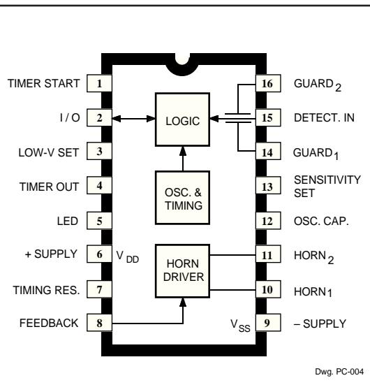
The A5349CA is a low-current, CMOS circuit providing all of the required features for an ionization-type smoke detector. A networking capability allows as many as 125 units to be interconnected so that if any unit senses smoke, all units will sound an alarm. In addition, special features are incorporated to facilitate alignment and test of the finished smoke detector. This device is designed to comply with Underwriters Laboratories Specification UL217.
