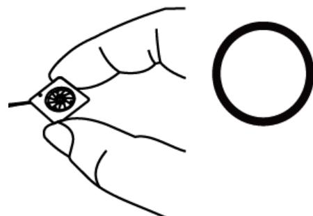
Don't pull fan with lead wires.
