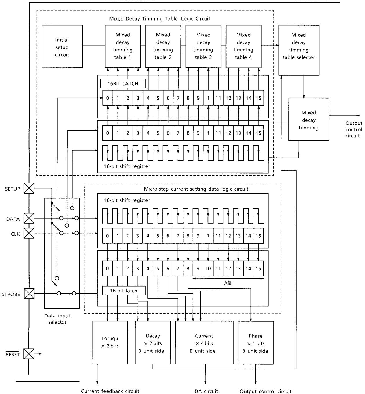
Note: The RESET and SETUP pins are pulled down in the IC by 10 kΩ resistor.
