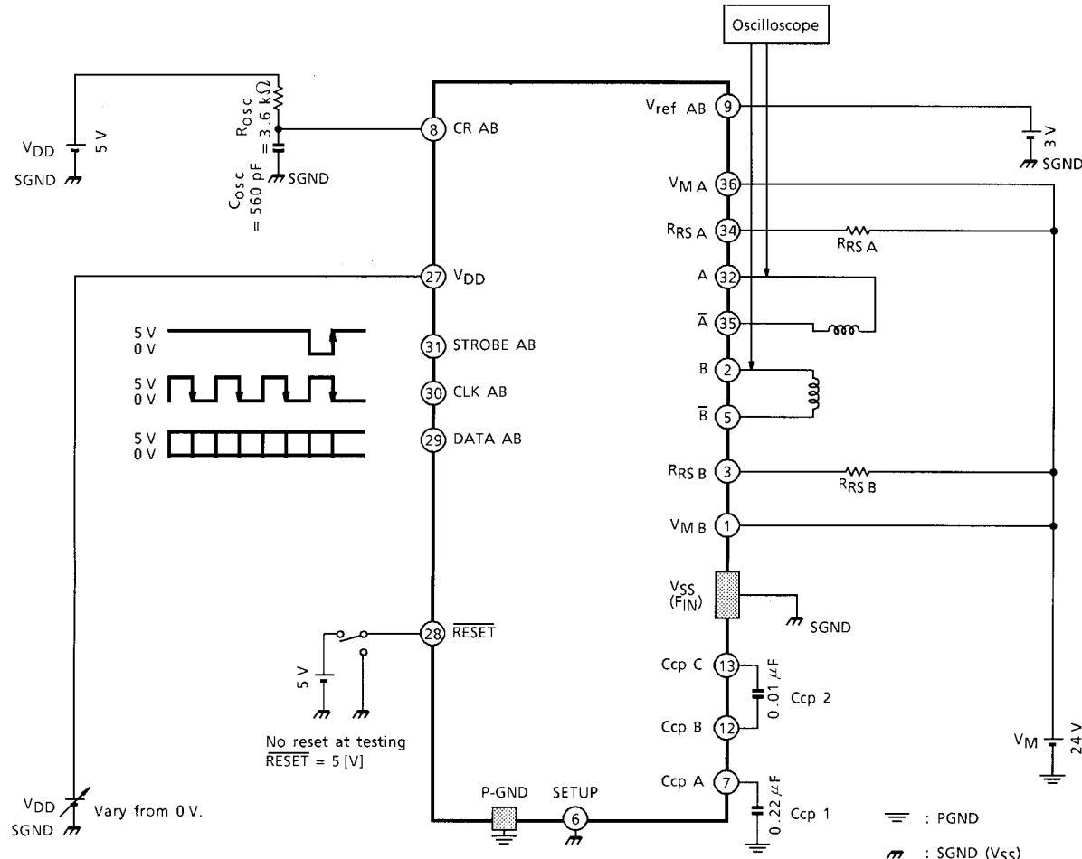
Monitor the output pins. Increase the V<sub>DD</sub> voltage from 0. Measure the V<sub>DD</sub> value when output starts. Next, decrease the V<sub>DD</sub> voltage and measure the V<sub>DD</sub> value when output stops.
