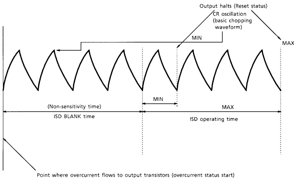
A non-sensitivity time is set for the overcurrent protector circuit to avoid misdetection of overcurrent due to spike current at irr or switching.
