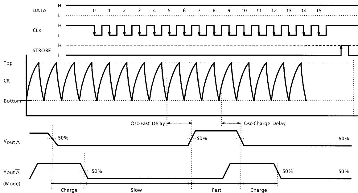
18.  $t_{pHl}$  (ST),  $t_{pLH}$  (ST),  $t_r$ ,  $t_f$  (A / B unit only. C / D unit conforms to A / B unit.)
