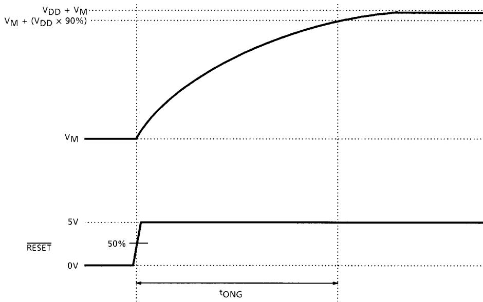
$t_{ONG}$ : Time taken for capacitor Ccp2 (charging capacitor) to fill up Ccp1 (capacitor used to save charge) to  $V_M + VDD$  after a reset is released.
