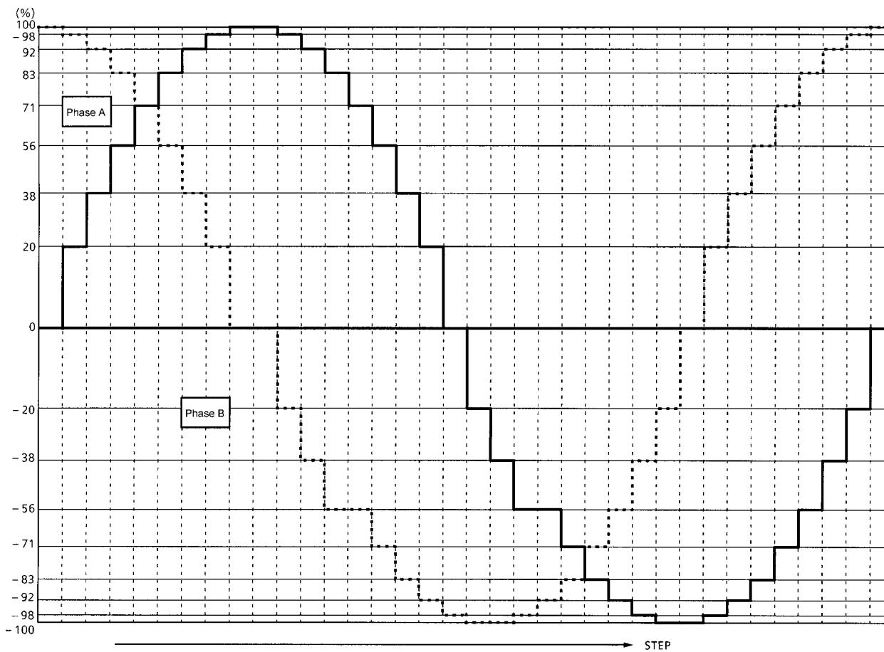
9 micro-step from 0 to 90° drive is possible by combining Current DATA (AB & CD) and phase data.
