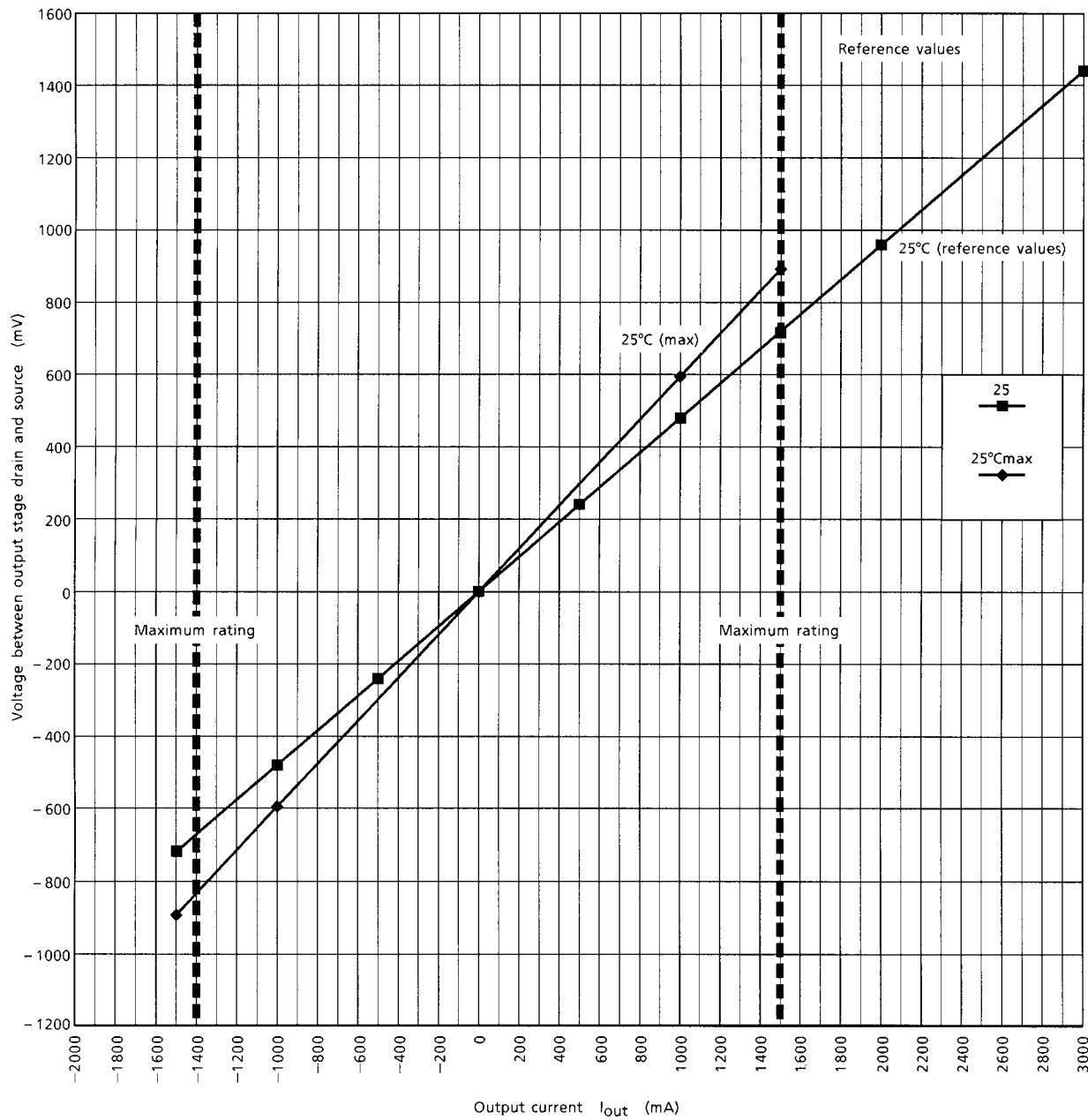
The IC's maximum rating is 1.5 A and recommended current is 1.2 A max.
