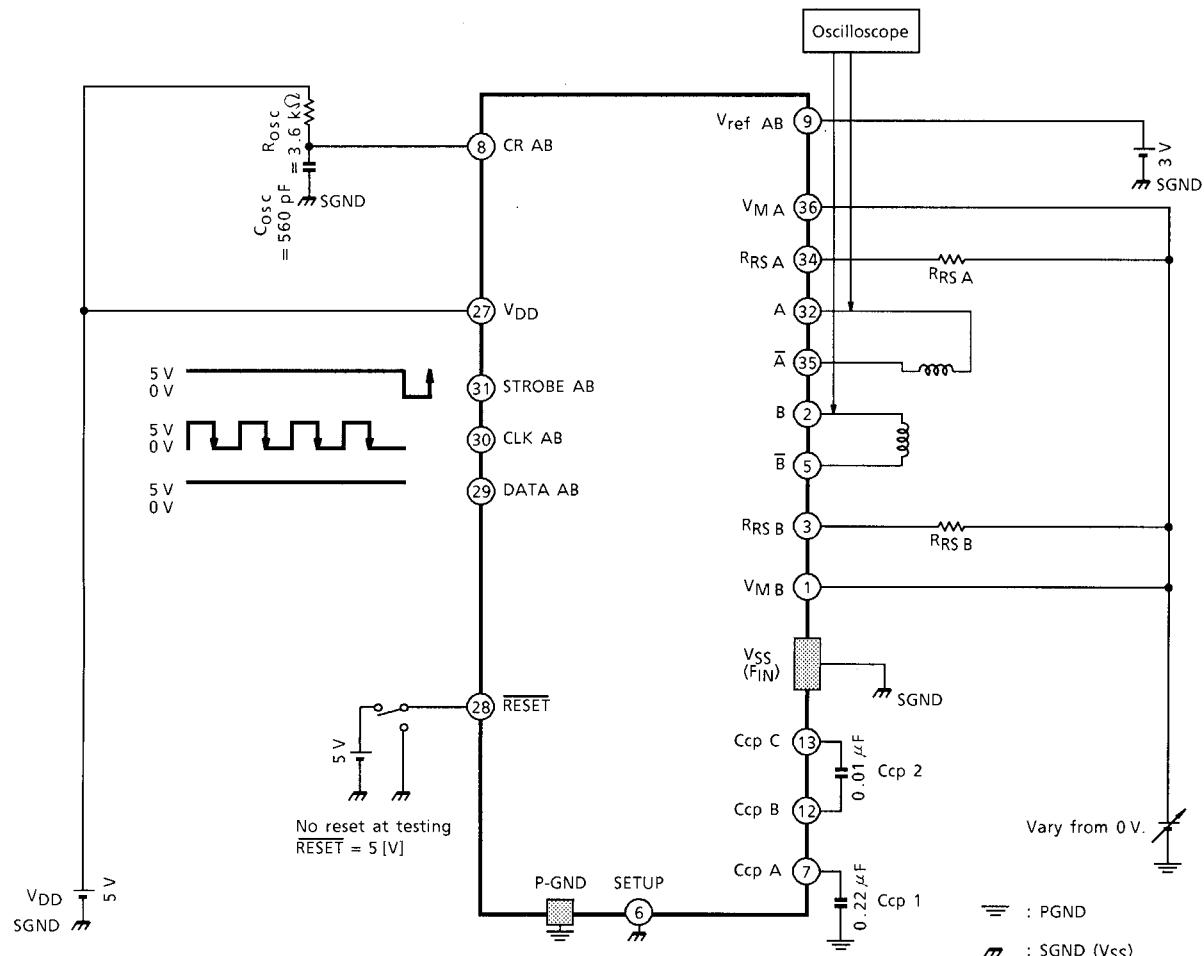
With the CLK signal and DATA (all High) input, increase the VM voltage from 0.
