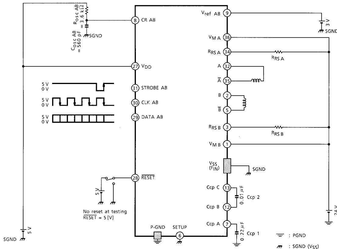
tBRANK is the dead time band for avoiding malfunction caused by noise. Apply sufficient differential voltage (when  $V_{ref} = 3\text{ V}, 0.6\text{ V}$  or higher) to  $VM-RS$  and apply duty. When the pulse width reaches a certain value, triggering feedback and changing the output. Check the value.
