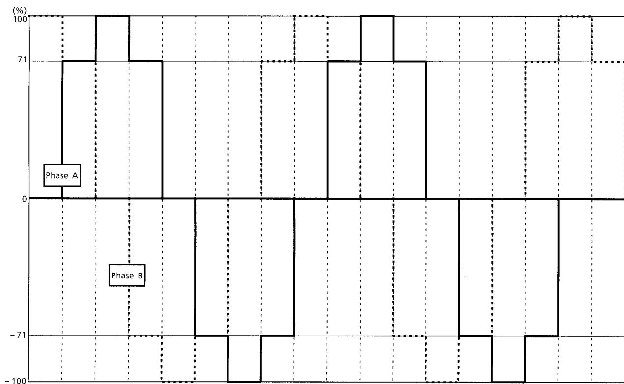
**APPLICATION OPERATION INPUT DATA (Example: 4-bit micro steps)**
