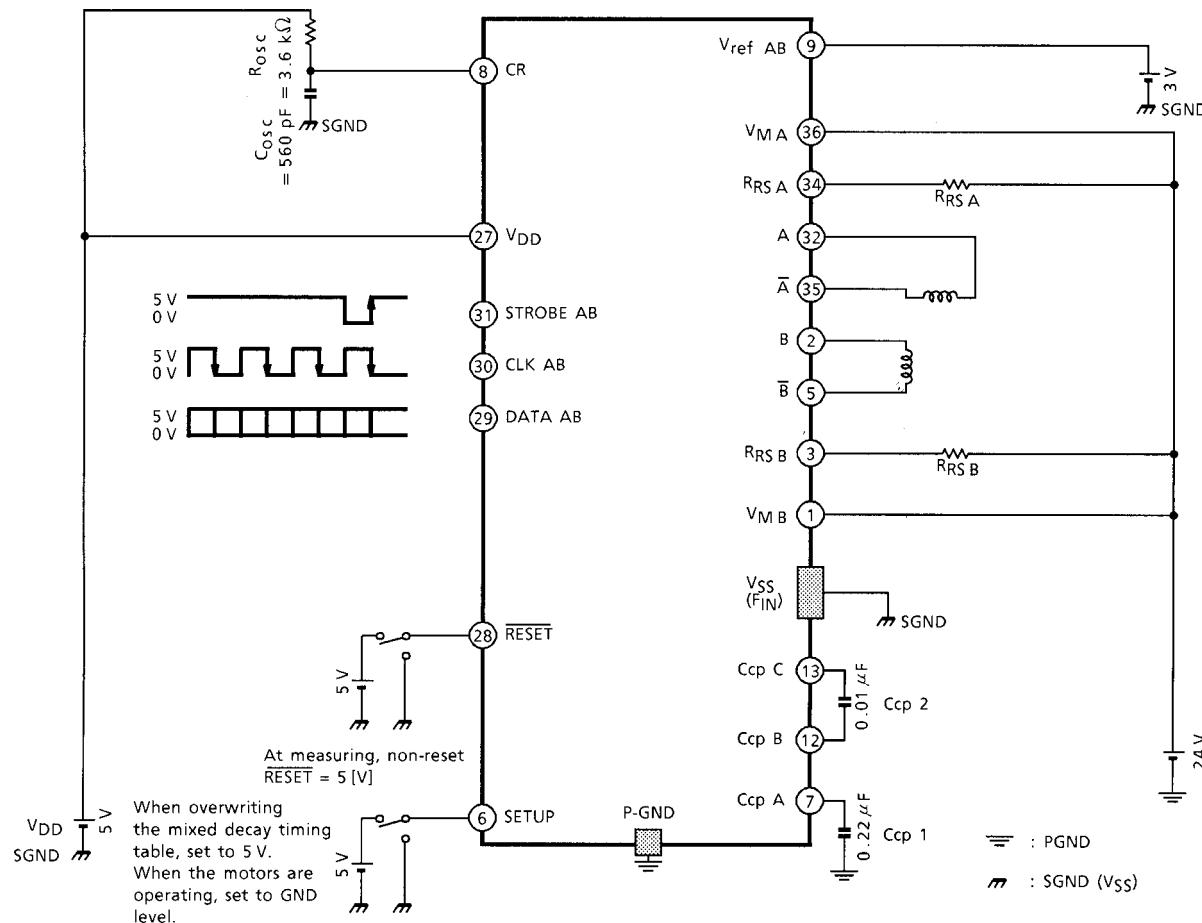
With  $V_M = 24$  V,  $V_{DD} = 5$  V,  $\overline{RESET} = H$ , change the SETUP pin from L to H and overwrite the MIXED DECAY TIMING TABLE.
