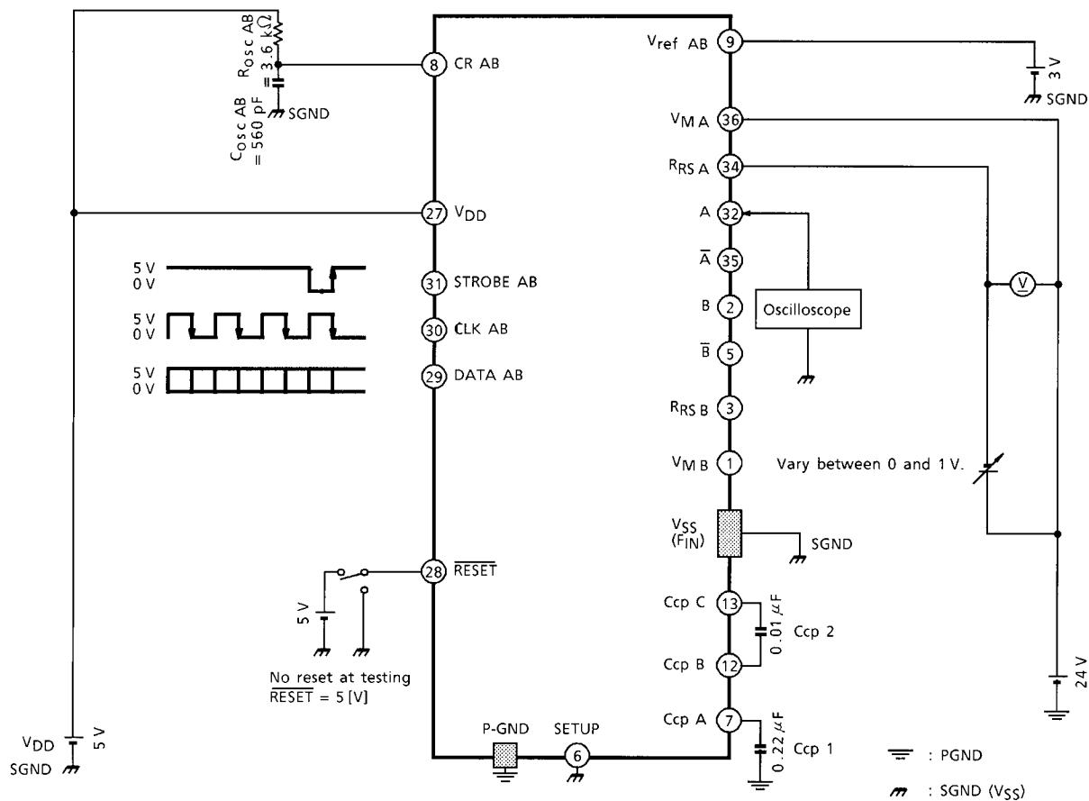
$V_{RS}$  (H~L): Input torque data = 100% (HH) and vary the voltage between  $V_M$  and  $R_S$  pins.
