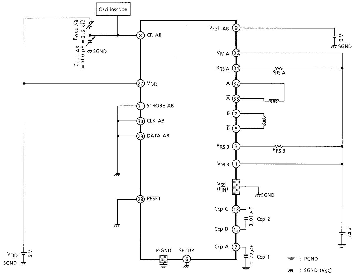
Change the  $R_{osc}$  and  $C_{osc}$  values and measure the frequency on the CR pin using the oscilloscope. At this time, 1 / 8 of the frequency of the measured CR waveform is  $f_{chop}$ .
