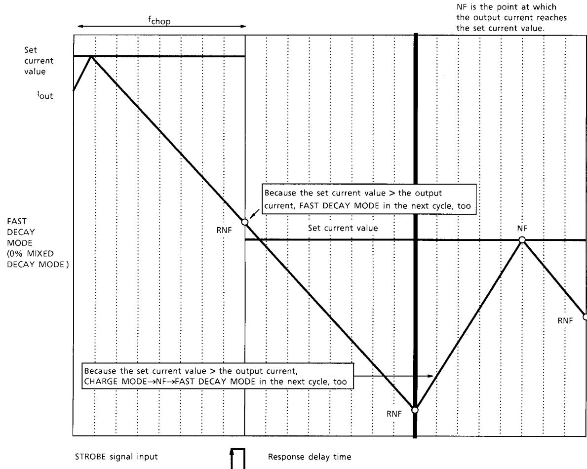
**STROBE SIGNAL, INTERNAL CR CLK, AND OUTPUT CURRENT WAVEFORM**
