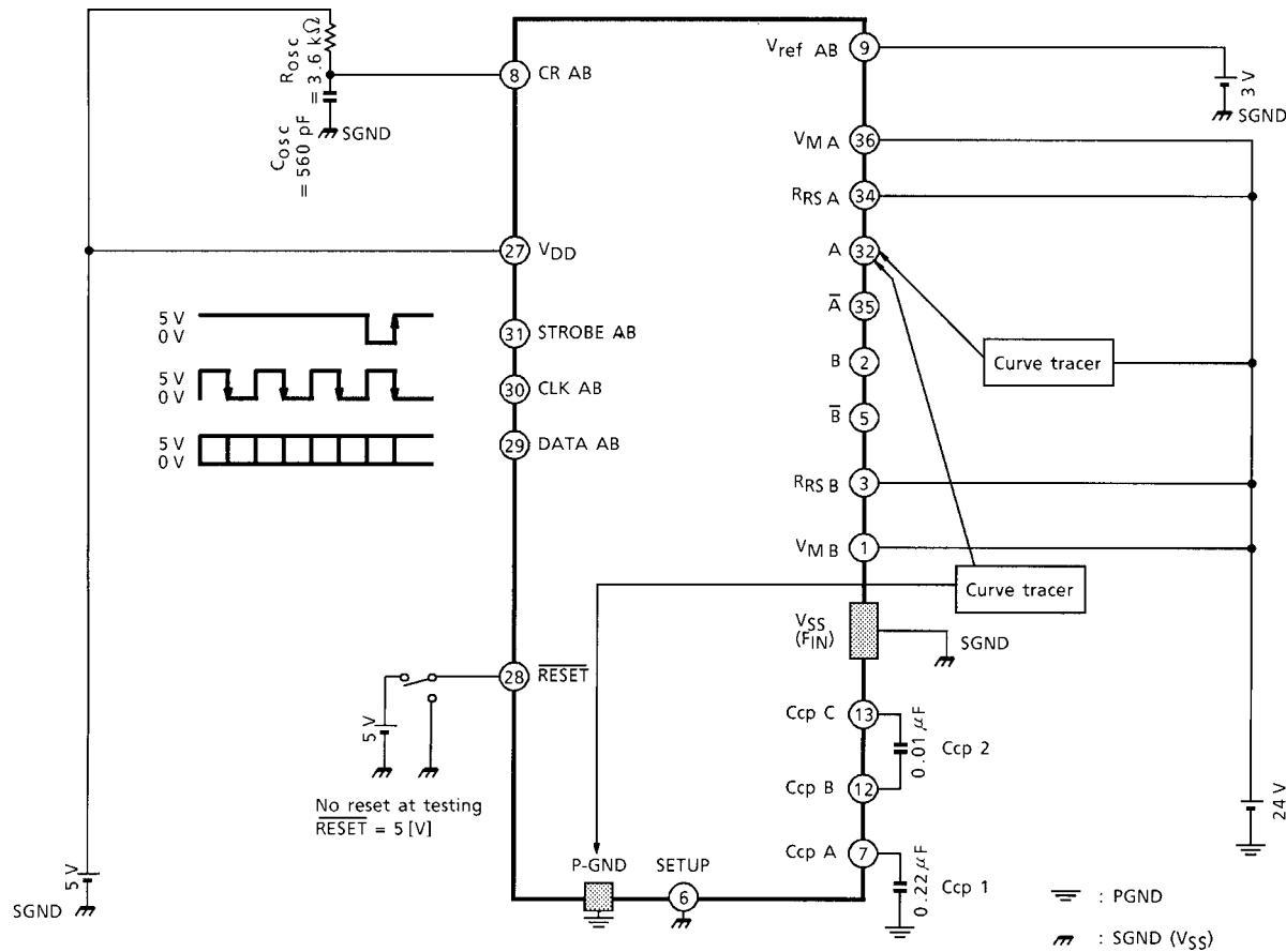
**T<sub>j</sub>TSD** : Increase the ambient temperature. Measure the temperature when output stops.
