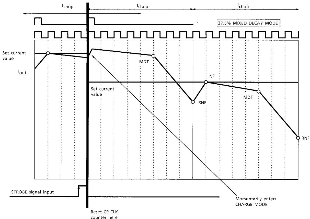
When STROBE signal is input, the chopping counter (CR-CLK counter) is forced to reset at the next CR-CLK timing.
