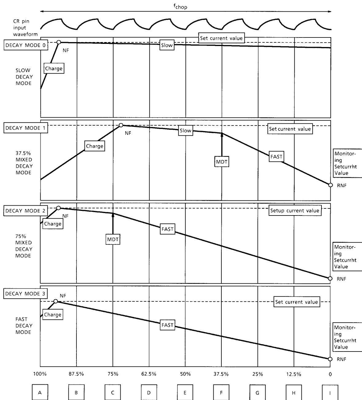
In Decay modes 1 to 4, any point from A to H can be set using 3-bit + 1-bit serial data  $\times 4$ .
