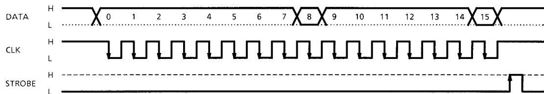
Test method: Set output to open, change phase data from  $1 \rightarrow 0 \rightarrow 1 \rightarrow 0$  and perform switching. When testing, input phase data at double the chopping frequency (if  $f_{chop} = 100$  kHz,  $f_{DATA} = 200$  kHz) and measure the current value of  $V_M$  supply.
