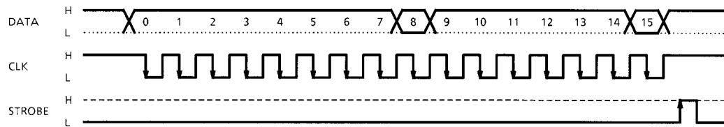
Switch PHASE every 130  $\mu\text{s}$  and measure the output pin voltage and the STROBE signal.
