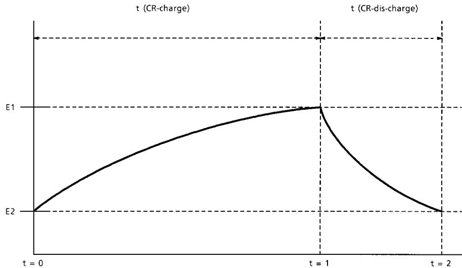
The OSC circuit generates the chopping reference signal by charging and discharging the external capacitor  $C_{osc}$  through current supplied from the external resistor  $R_{osc}$  in the OSC block.
