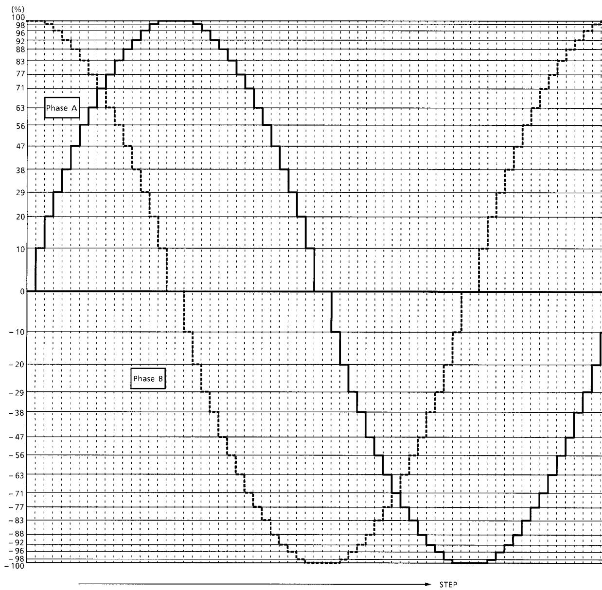
17 micro-step from 0 to 90° drive is possible by combining Current DATA (AB & CD) and phase data.
