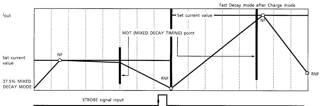
In MIXED DECAY MODE, when the output current > the set current value
