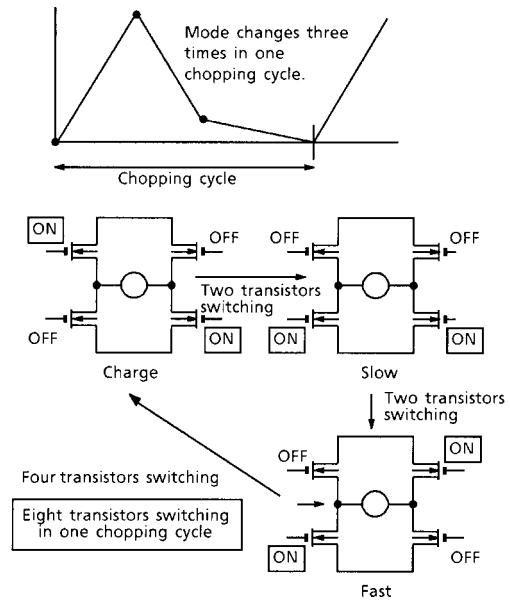
Number of switchings at actual operation =  $2 \times$  number of switchings at phase switching.
