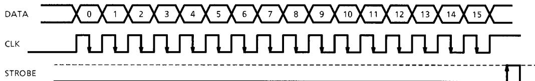
Note: Data input to the DATA pin are 16-bit serial data.
