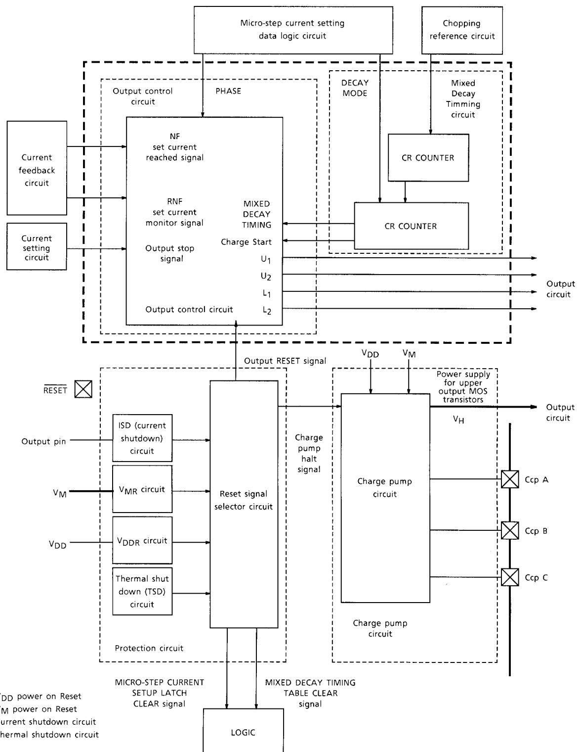
Note: The RESET pins is pulled down in the IC by 10-kΩ resistor.
